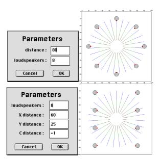
Figure 3: Automatic speaker placement in Holophon (top: circular, bottom: lateral).
