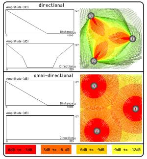
Figure 2: Left: loudspeaker response tables Right: levels curves of the speakers in relation to the tables.
